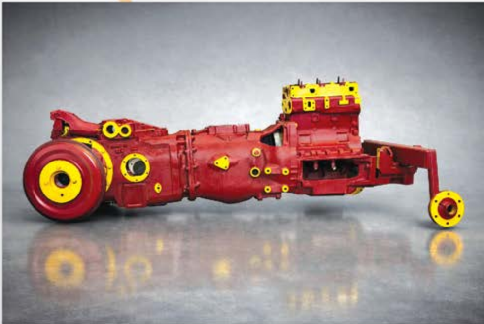
MF-240 Tractor Chassis Made from BCL Castings
